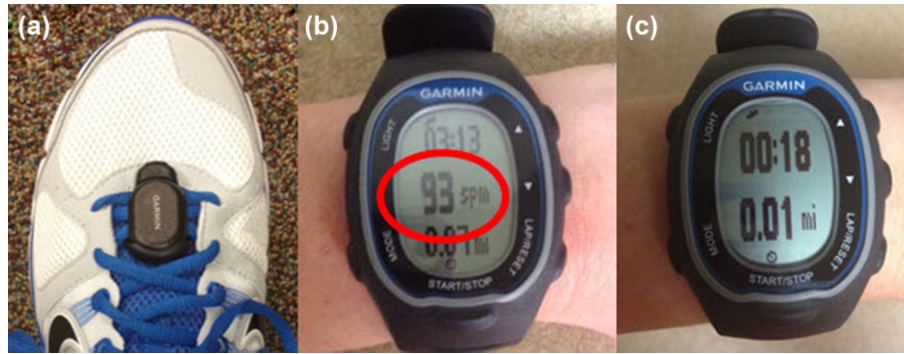
Fig. 1. The Garmin FR70 that was used for all retrainers and controls: (a) A wireless accelerometer transmitted data to the wrist-mounted running computer. (b) The wrist-mounted running computer was configured such that running duration, real-time strides per minute steps per minute divided by 2 and running distance were visible to all retrainers during in-field retraining sessions 1–3, 5, and 7. (c) During in-field retraining session 4, 6, and 8, retrainers were only able to view feedback on run duration and distance run as step rate feedback faded. All control subjects only viewed the display in (c).
